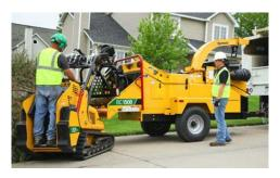
**ENGINE OPTIONS.** The BC1500 is offered in either a 165 hp (123 kW) PSI 5.6L gasoline engine and 130 hp (97 kW) Cummins QSF 3.8L Tier 4 Final engine.
