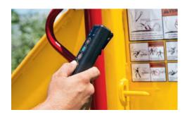
**TAKE CONTROL.** With the optional Tree Commander<sup>™</sup> remote control, jobsite productivity can be improved by allowing the operator to control brush chipper functions remotely. The remote can be attached to the operator's belt or held in an optional bracket mounted directly to the operator's station of a Vermeer compact utility loader.
