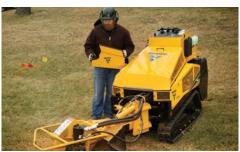
CHOOSE YOUR VIEW. The side operator's station offers the ability to select the best angle from which to view the stump during operation and provides all control functions for cutter wheel and ground drive creep forward and reverse.
