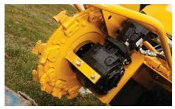
ON THE CUTTING EDGE. The cutter wheel is equipped with Vermeer proprietary Pow-R<sup>™</sup> plate technology which helps to lessen bounce while cutting, increase protection of cutter tooth pockets and reduce horsepower robbing chip recirculation.
