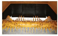
**DURABLE WEAR ZONES.** Machine tunnel is built with .25" (6.4 mm) steel plates to help protect and extend the life of the high wear zone.
