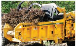
PROGRESSIVE PROCESSING. The patented SmartFeed system monitors engine rpm and adjusts grinding speed to increase productivity. The open-ended, wide infeed table makes material loading easy and efficient.
