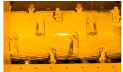
**OPTIMAL CUTTING PERFORMANCE.** The new Series III duplex drum is built off the proven cutting performance of previous Vermeer duplex drum designs, and makes maintenance more convenient with enhancements such as an independently secured wedge system and enhanced drum balancing.
