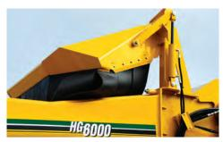
JOBSITE SAFETY. The thrown object deflector (TOD) reduces the amount and distance of thrown material debris, while also reducing interference when loading over-length material.
