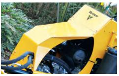
**MINIMIZE SERVICE TIME AND TOOLS.** You know serviceability isn't an option. The engine cover design offers virtually "no-tool" access to all daily and weekly service points, making for quick service turnaround.
