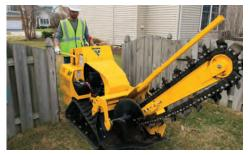
**SLENDER PROFILE DESIGN.** A 34.5" (87.6 cm) width helps the unit fit through tight areas and narrow gates.
