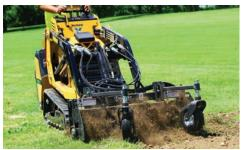
**BUILT TO PERFORM.** Get more out of each day with a rated operating capacity of 925 lb (419.6 kg) while reaching to maximum hinge pin height at 85.5 in (217.7 cm).
