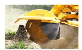
PATENTED SMARTSWEEP™ CONTROL **SYSTEM.** The patented SmartSweep control system monitors engine speed and automatically adjusts cutter wheel sweep rate to maximize power to the cutter wheel while reducing engine stress.
