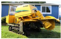
TRACTIVE EFFORTS. The SC70TX is equipped with an increased ground drive speed and is designed with a track to help decrease ground disturbance.
