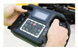
**OPTIONAL REMOTE CONTROL.** An optional remote control allows operators to maneuver the stump cutter while away from the unit.
