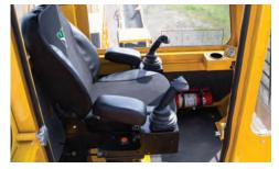
CONTROL IN YOUR HANDS. The loader's electric-over-hydraulic controls provide the flexibility for an operator to use their preferred control configuration (Vermeer, SAE or ISO), as well as three operating modes with varying joystick sensitivity to meet the operator's needs.
