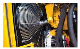
**OPERATING EFFICIENCY.** With features such as a hydraulically actuated variable flow and reversing Flexxaire cooling fan, the TG5000 is built with operating efficiency top of mind. The fan adjusts the pitch of the blades based on temperature, which can increase the power available to the mill for better processing efficiency. Vermeer
