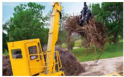
JOB EFFICIENCY. An optional loader cab with grapple increases efficiency and can lift up to 3500 lb (1587.6 kg) at full reach.
