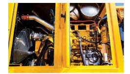
**ENGINE POWER.** The TG5000 is powered by a 540 hp (403 kW) Caterpillar C15 Tier 4 Final engine, with a maximum fuel consumption of 27 gal/hr (102 L/hr). A 540 hp (403 kW) Tier 3 engine option is available for lesser-emission regulated countries.
