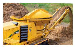
JOBSITE SAFETY. The patented Thrown Object Restraint System (TORS) reduces the amount and distance of thrown objects, and has a smooth underside for better material flow.
