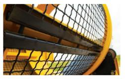
**PRODUCT VARIETY.** Change product size more efficiently with the quick-change screen design. Five large bolts adjust a tensioning hook to allow operators to quickly change screen sizes.
