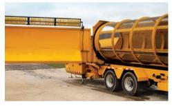
**DRUM SERVICE ACCESS.** A single-hinged side panel exposes the full length of the trommel drum from ground level for drum service and removal.
