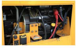
**ENGINE.** The TR6400 features a Deutz 3.6L Tier 4F (Stage IV), 100 hp (75 kW) engine. The engine is mounted on a pivoting frame that swings out 30 degrees for access to fuel filters and hydraulic reservoir for maintenance and service.
