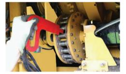
**DRUM DRIVE.** A hydraulic chain drive system allows the drum to lift off the cog for service. Bolt-on sprockets can be changed quickly and help minimize repair.
